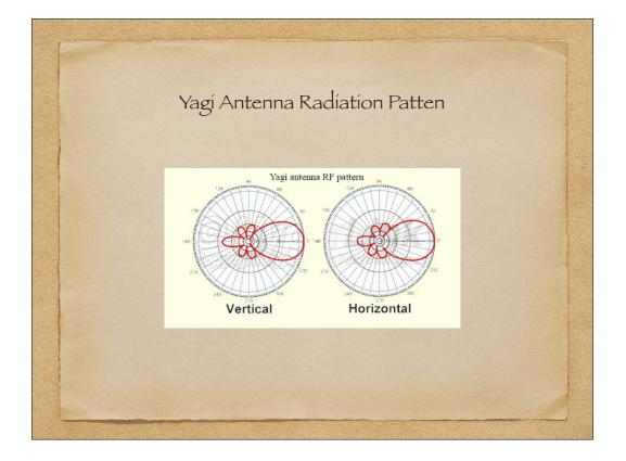
To focus the beam in the vertical: add elements to the beam To focus the beam in the horizontal: stack another yogi
