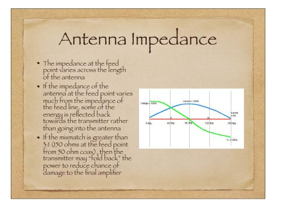
The method to address the mismatch is to insert a "transmatch" (short for transformer match) between the feed line and the antenna
