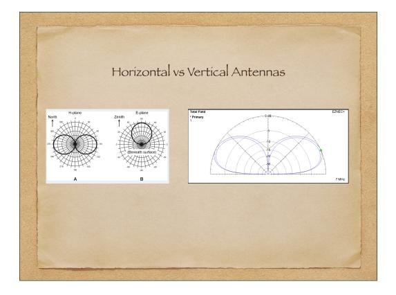
Vertical antenna has a lower take-off angle
