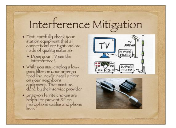
High-pass filter: allows high frequencies to pass, attenuates frequencies below the cut-off frequency.
