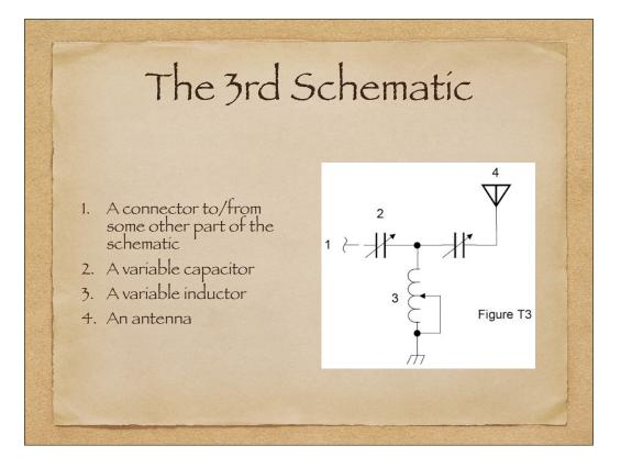
This circuit actually works, whereas the other two circuits are pretty much nonsense. This circuit is a trans match to make the transmitter think it's seeing a 50 ohm impedance.
