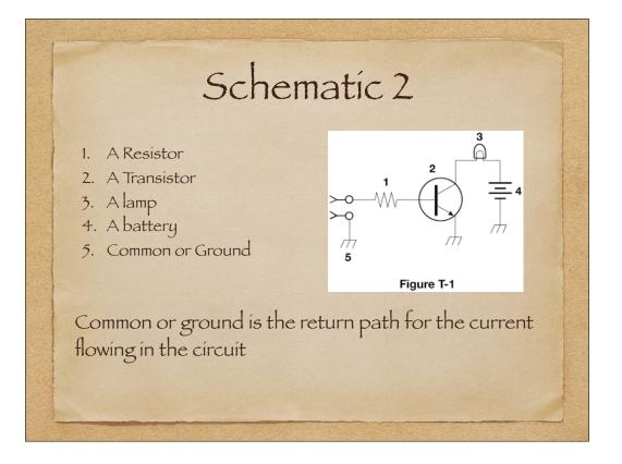
The only thing this circuit does is turn on a lamp if some other part of the circuit (which isn't shown) draws current.
