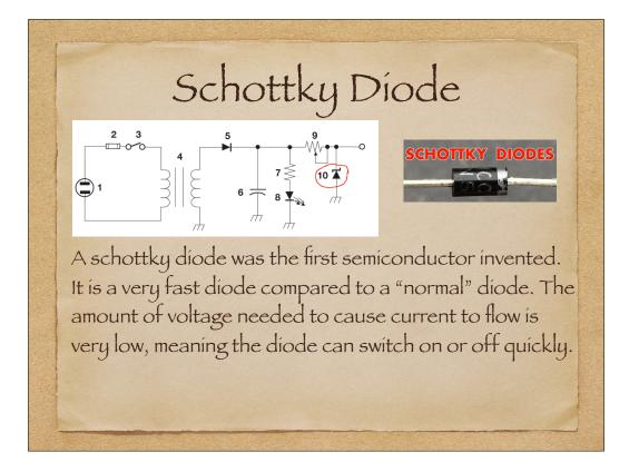
The Schottky Diode is distinguished from "normal" diodes by the "curly" cathode indicator. Note that in a Schottky Diode, the current flows from the cathode to the anode whereas in normal diodes, current flows from the anode to the cathode (compare #5 to #10)
