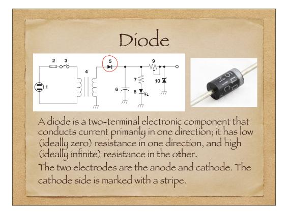
Current flows from the anode to the cathode. Diodes have a threshold voltage value and current will flow when the threshold is exceeded.
