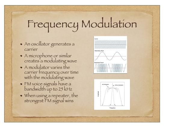
**Frequency deviation** is used in FM radio to describe the maximum difference between an FM modulated frequency and the nominal carrier frequency. The width of an FM signal varies as the carrier is modulated. The amount of variation in the width is call "deviation". If the fully modulated signal "deviates" more that 25 kHz, it is over deviating. Usually that is caused by talking too loudly into the microphone or holding the microphone too close to the mouth.
