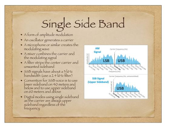
When SSB was beginning to be implemented, the circuitry to filter out the unwanted sideband made it fairly easy to generate a lower sideband signal for transmitted signals below 50 meters and to easily generate an upper sideband signal for transmitted signals above 50 meters. In today's solid-state transmitters, that's no longer the case, but the convention remained.
