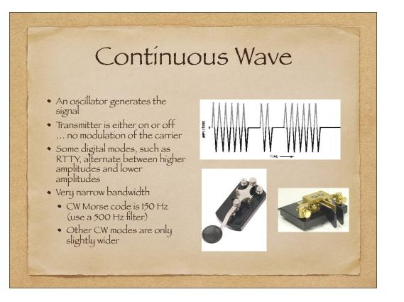
Signal to Noise Ratio: One way to improve the SNR is to narrow the bandwidth of the received signal. A CW signal carrying morse code is about 150 Hz wide. If the receiver is receiving a bandwidth of 6 kHz (the width of an AM broadcast signal), there is a lot of unwanted noise surrounding the CW signal. Most modern transceivers have a set of filters of various widths that can be switched in to narrow the received bandwidth thus making the desired signal more prominent.
