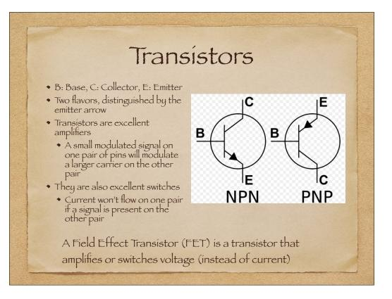
When input voltage applied to Base/Emitter, it changes the resistance between the Collector and Emitter. That then affects how much current can flow between the Collector and Emitter
