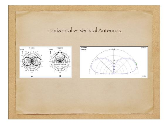
Vertical antenna has a lower take-off angle
