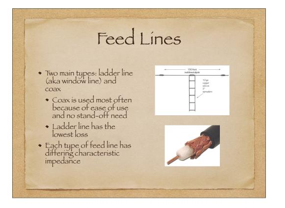
The antenna connector on the back of the transmitter / receiver expects to see an impedance (resistance) of 50 ohms Coax generally has either 50 ohms or 75 ohms of impedance (50 ohms ... amateur; 75 ohms ... TV)
