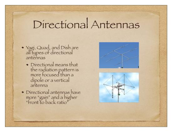
Gain: a process of taking RF energy and focusing it in an intended direction
